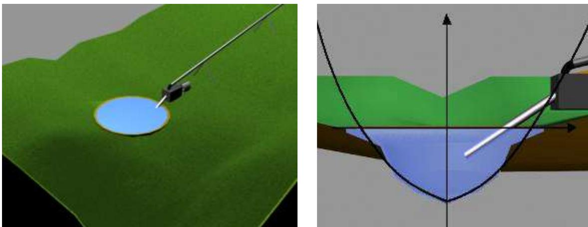
Figure 2 – Approximate parabola of the dam.
