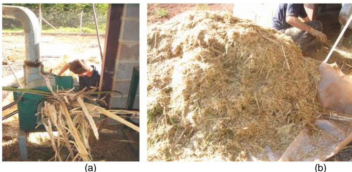
Figure 3. Chopping process (a) Processing in Nogueira DPM-2 hammer mill, (b) chopped sugarcane
