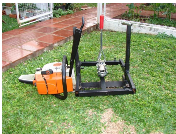
FIGURE 4. BUILT PORTABLE SAWMILL
