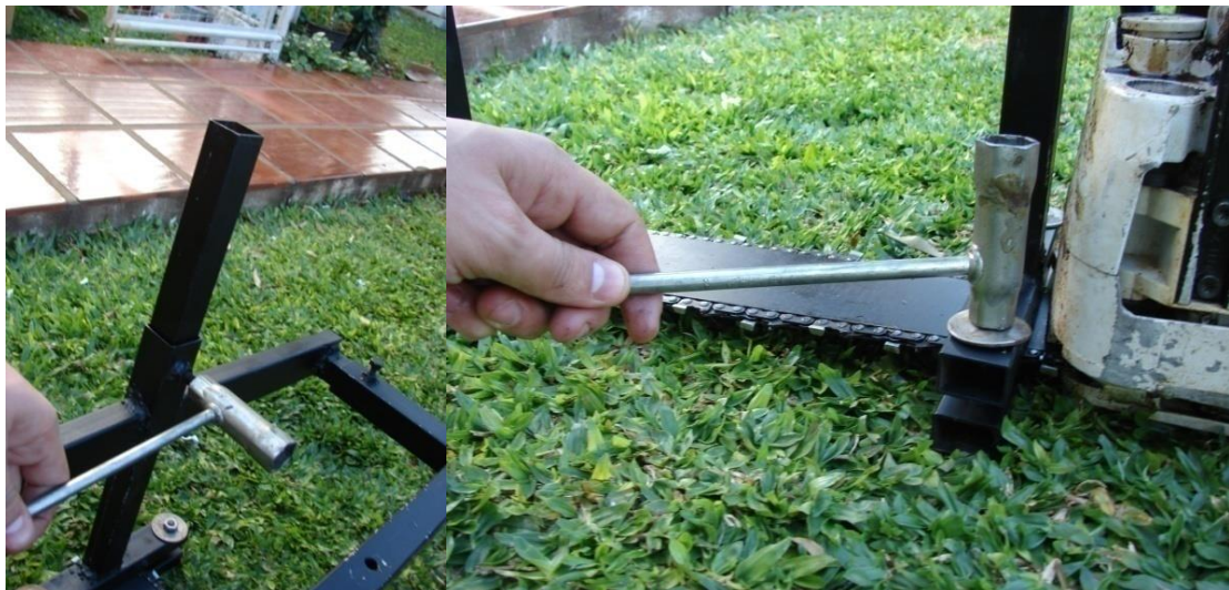
FIGURE 2 AND 3. ORIGINAL CHAINSAW TOOL CLAMPING THE SCREWS
